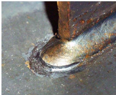
Figure 2-5: Impact treatment and geometry improvement of a weld toe (Dexter & Ocel, 2013)
